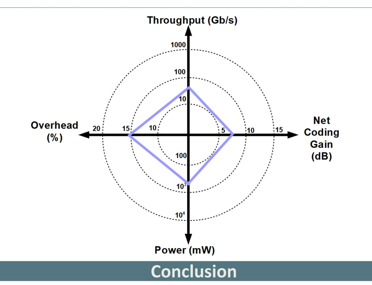
We demonstrate an end-to-end system of list-of-two SC decoder. System operates at 65 MHz clock frequency on FPGA. The FPGA implementation results show that the decoder IP Core exceeds 50 Gb/s throughput under 9.84 pJ/b energy efficiency with a coding gain of more than 7dB at 10<sup>-13</sup> BER relative to uncoded transmission.
