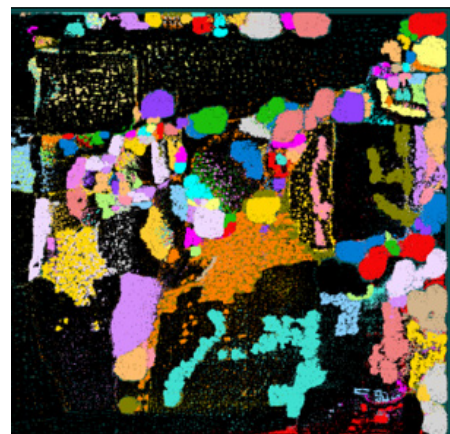
Layout of an 512/427 polar code list decoder with list size 2 in 28nm technology that outperforms state-of-the-art with 17x higher throughput, 10x higher area efficiency and better energy efficiency.
